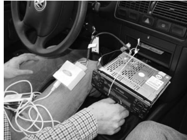
You will need to remove the factory radio to connect a factory iPod adapter to your car stereo.
