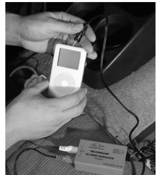
Use a mini-jack-to-RCA cable to connect your iPod to the FM modulator.
