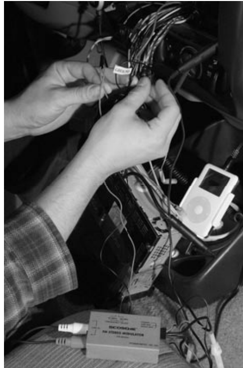
You can tap power and ground for a wired FM modulator from the car radio wiring harness.
