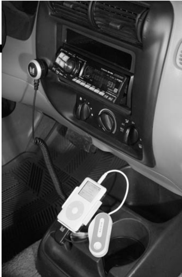
A wireless FM transmitter plugs into the iPod's headphone jack.
