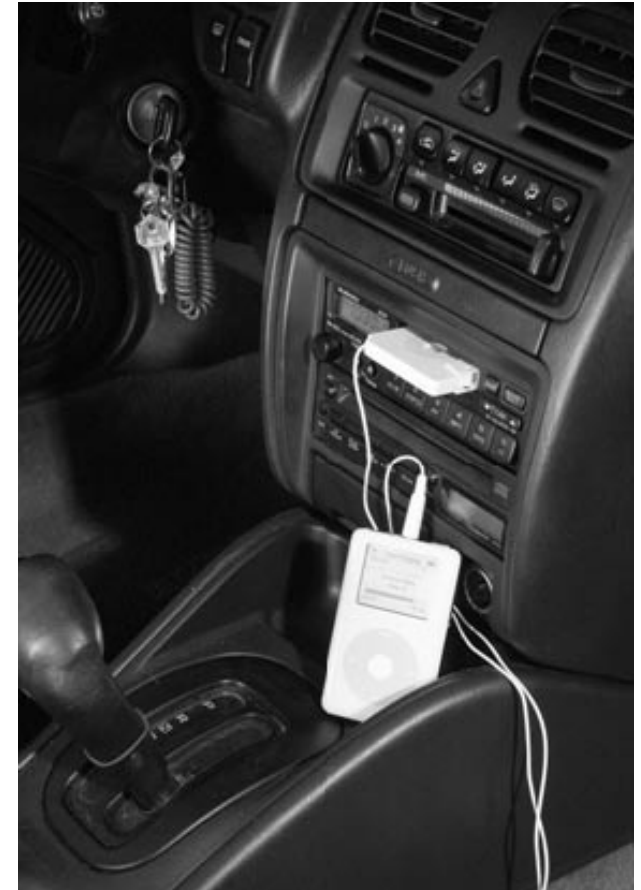
A cassette adapter remains a popular way to play an iPod through a car stereo.
