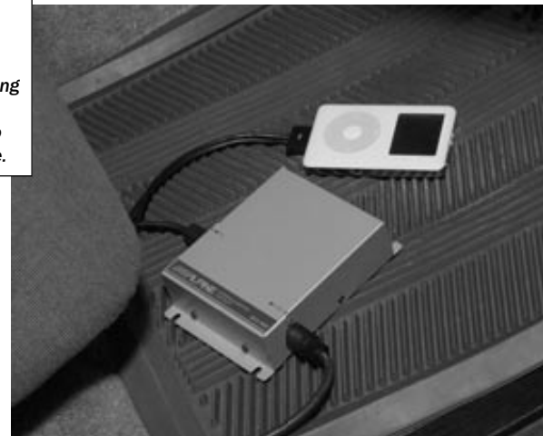
A brand-name radio iPod adapter connects to your radio's CD changer port and the iPod.
