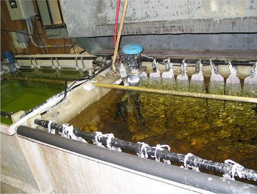
This is the silver tank. All instruments to be silver plated are submerged in this tank. Electricity then makes the silver molecules stick to the instrument. Notice the solid silver bars on the sides of the tub.
