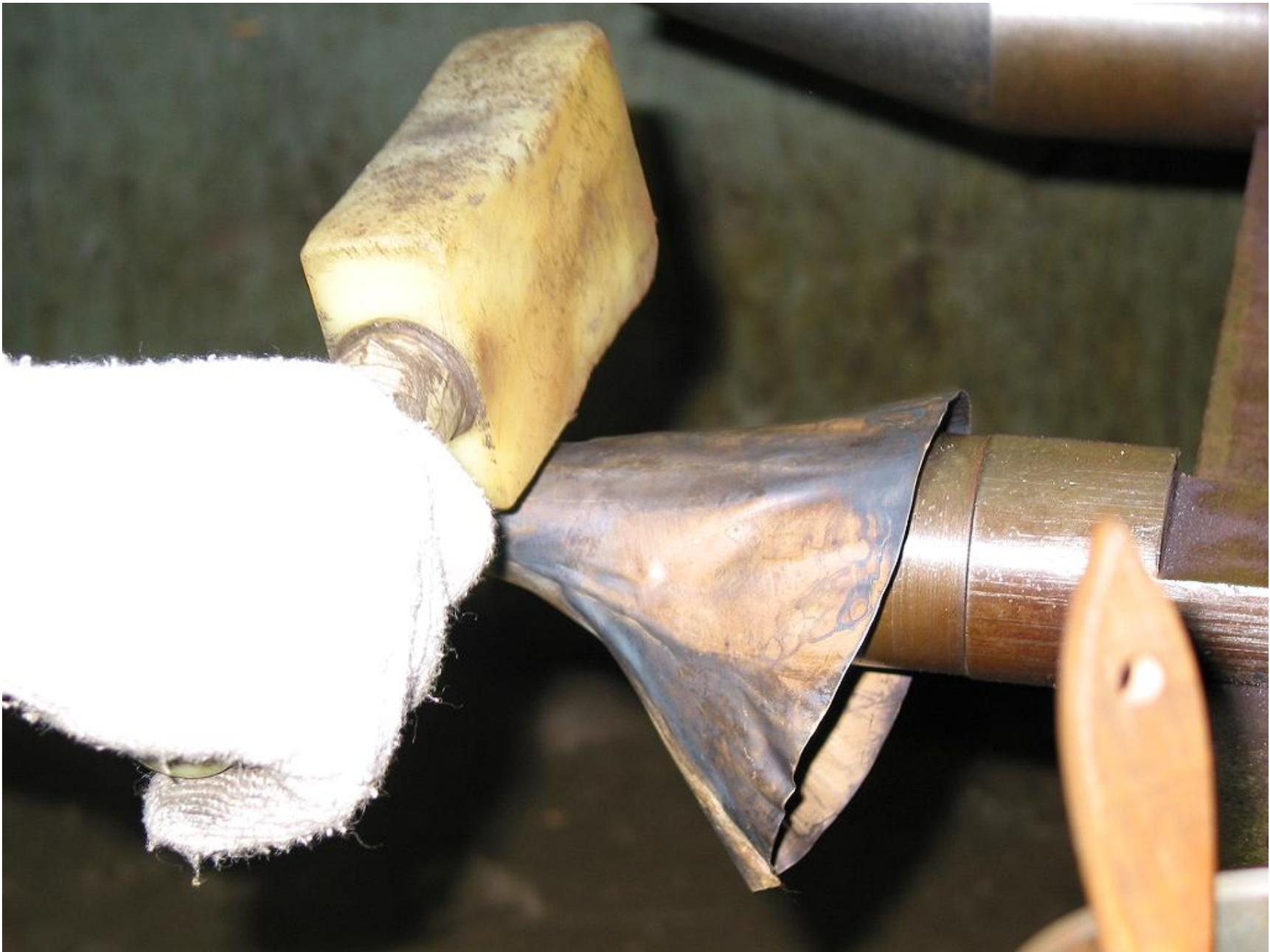
Using a soft mallet to give the bell its initial shape.
