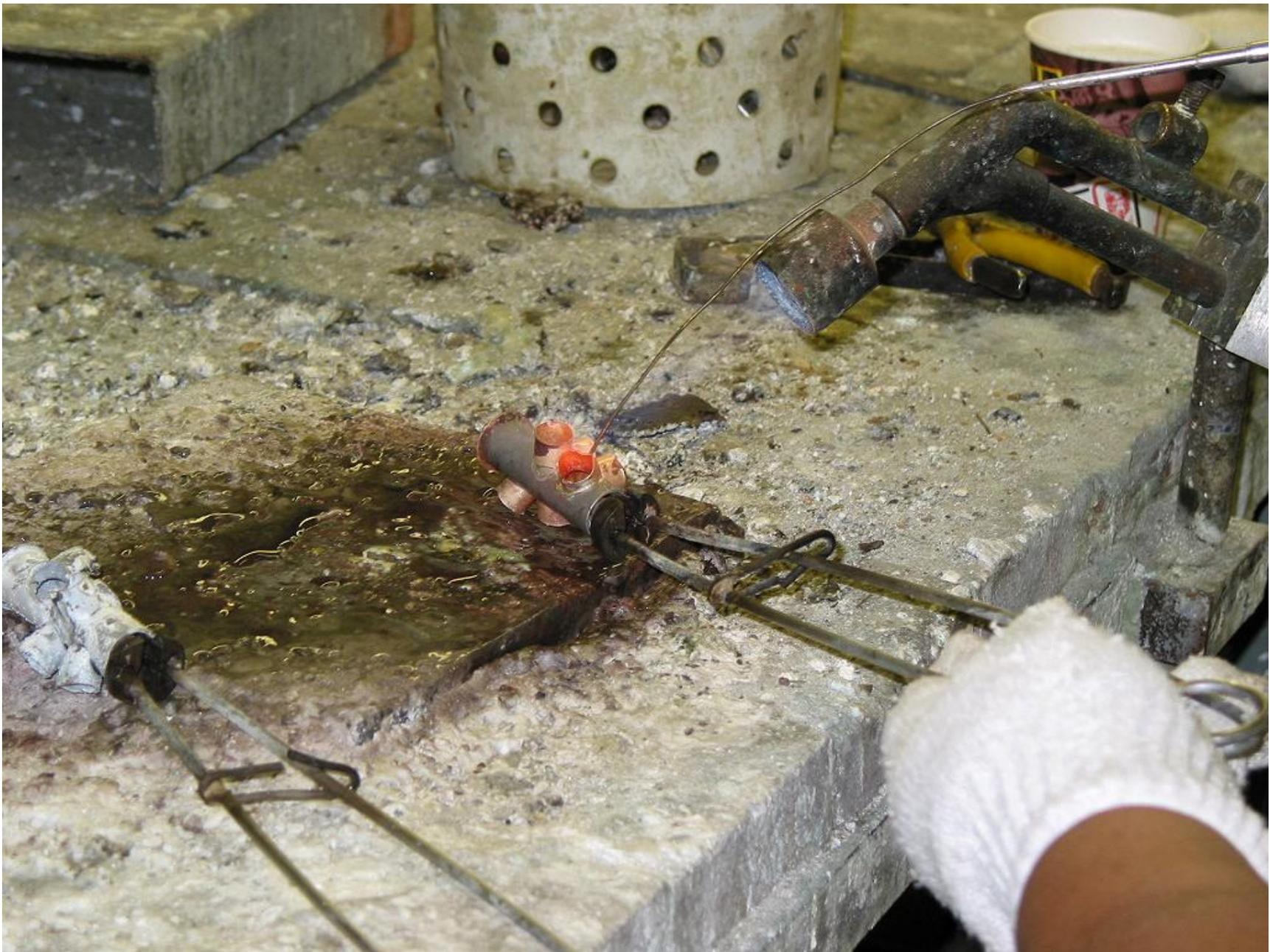
Soldering on the knuckles to the valve casing. The metal must become red hot for the silver solder to flow. It will then be a permanent structure.
