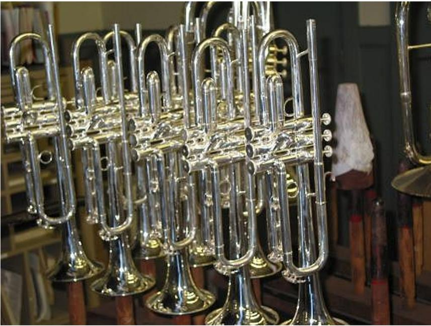
Silver plated trumpets that have been fitted with valves and slides. They are now ready for inspection and play testing.
