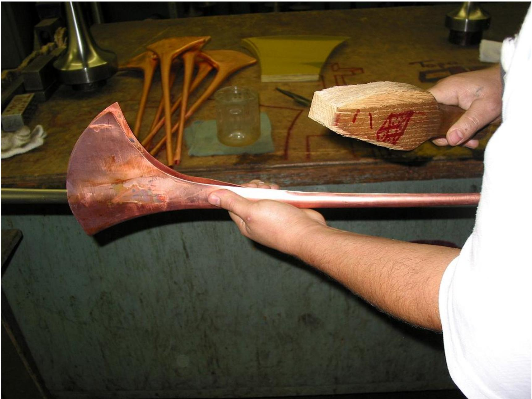
The material is hammered so it bends around. The two edges must come together and actually overlap, in order that they can be joined permanently. The two edges are then heated red hot and soldered together. The bell is soldered with a brass solder, which is yellow in color. This makes a yellow line which is invisible on Brass bells but really shows up on Copper bells because of the color contrast.
