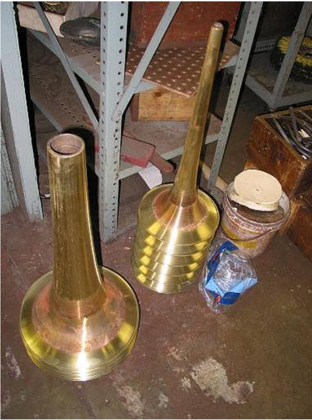
These bells have just been hand spun on the spinning lathe.
