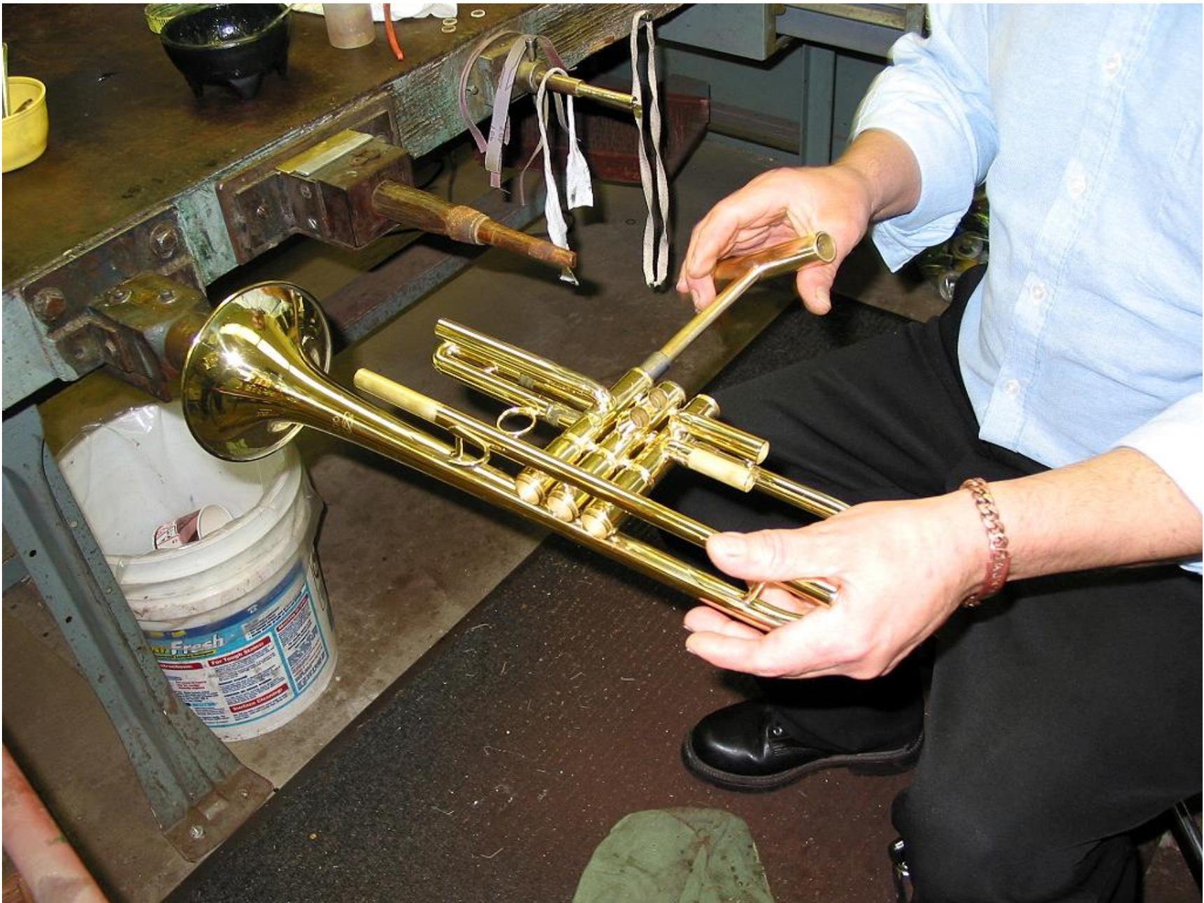
Lapping the valves. He screws a handle onto the actual valve that will go into that casing. He then spreads lapping compound on the valve and moves the valve back and forth in the casing until its a perfect fit is created. Lapping compound is just sand paper in a paste form. If he does not lap it enough the valves will be too tight, if he over laps it, the valves will be loose as a goose and leak air.
