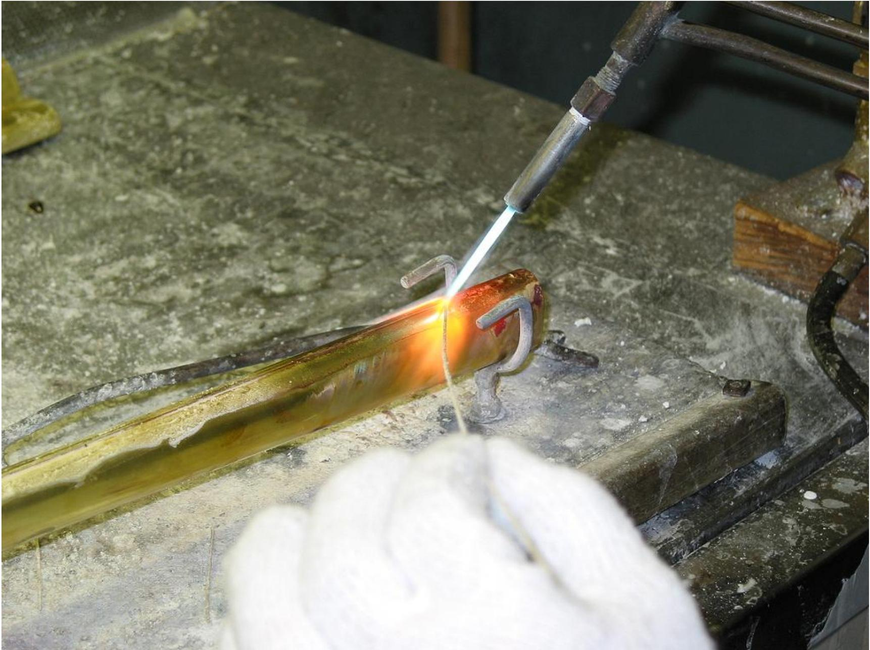
Ever wonder why you can see the seam on a copper bell. Because its made of sheet metal and brazed together with a brass alloy to form a tapered tube. I always liked the look of that seam. You can really see how the thing
