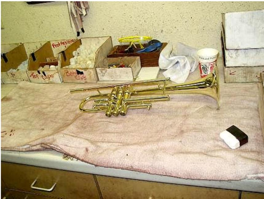
Lacquered instruments ready for valve fitting and assemble.
