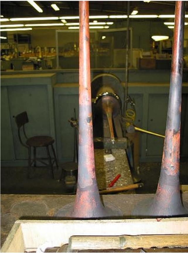
Bells that have just been spun by the lathe in the background. The discoloration is due to the annealing process.
