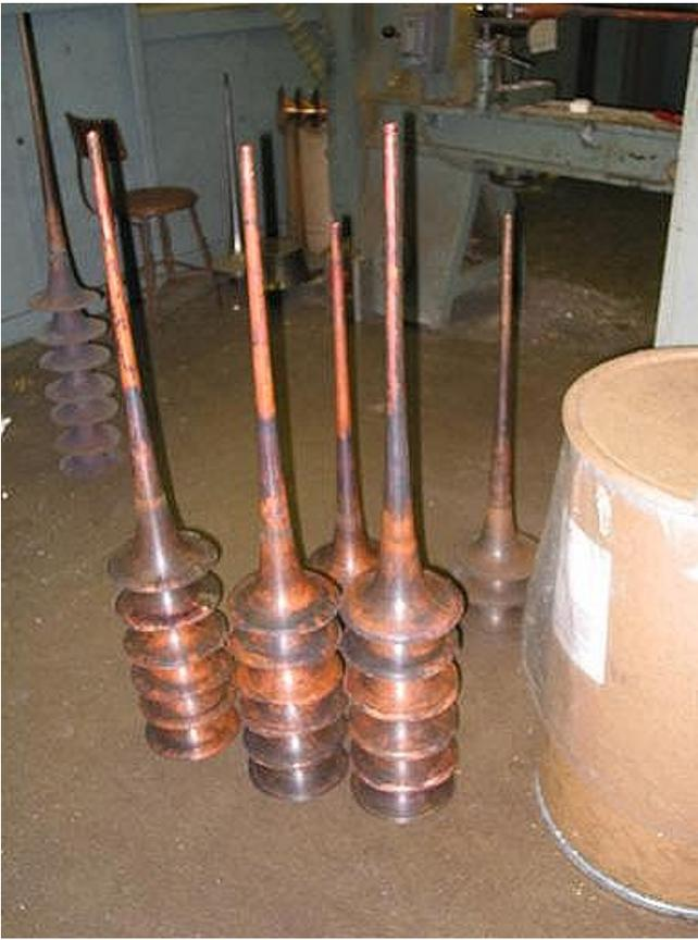
Spun single piece bells ready to go to the bending machine to have the crooks bent into a U shape.
