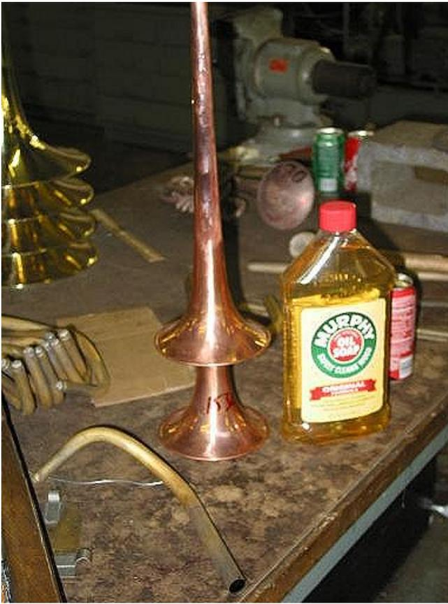
Something very interesting, the inside of smaller tubes such as the bend of a trumpet bell stem is filled with a mixture of water and soap. This is used because a soapy mixture will not freeze as hard and will not expand as much as pure water. This ensures that the thin walls of the tubes will not crack or split.
