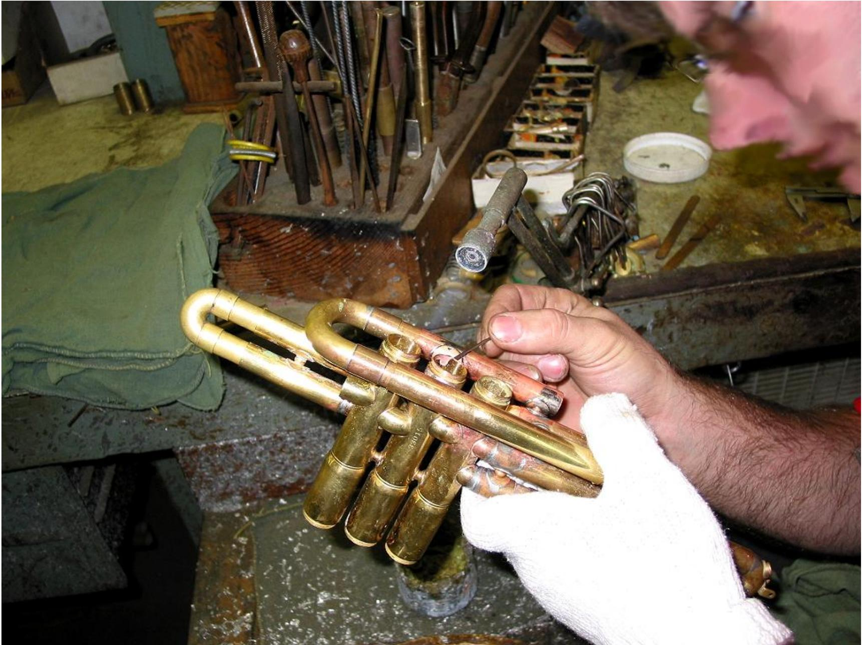
Assembling a horn is a messy job, everything actually has to align perfectly. If you look carefully, you will see the torch is on and the brace is being sift-soldered to the valve section. This person actually holds a very important position at the factory doing and overseeing many jobs. Identity concealed at his request.
