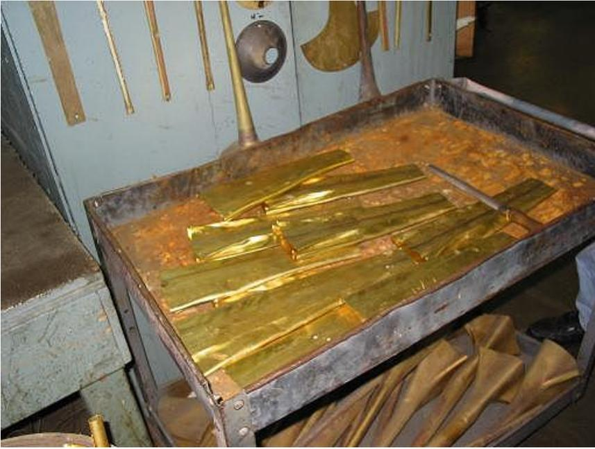
On the top shelf you see sheet brass cut to shape and soldered into a tube. Just below you see the next step of hand forming this sheet metal to a shape that barely resembles a bell. The bell spinners are the ones that finish the bell as we know it.
