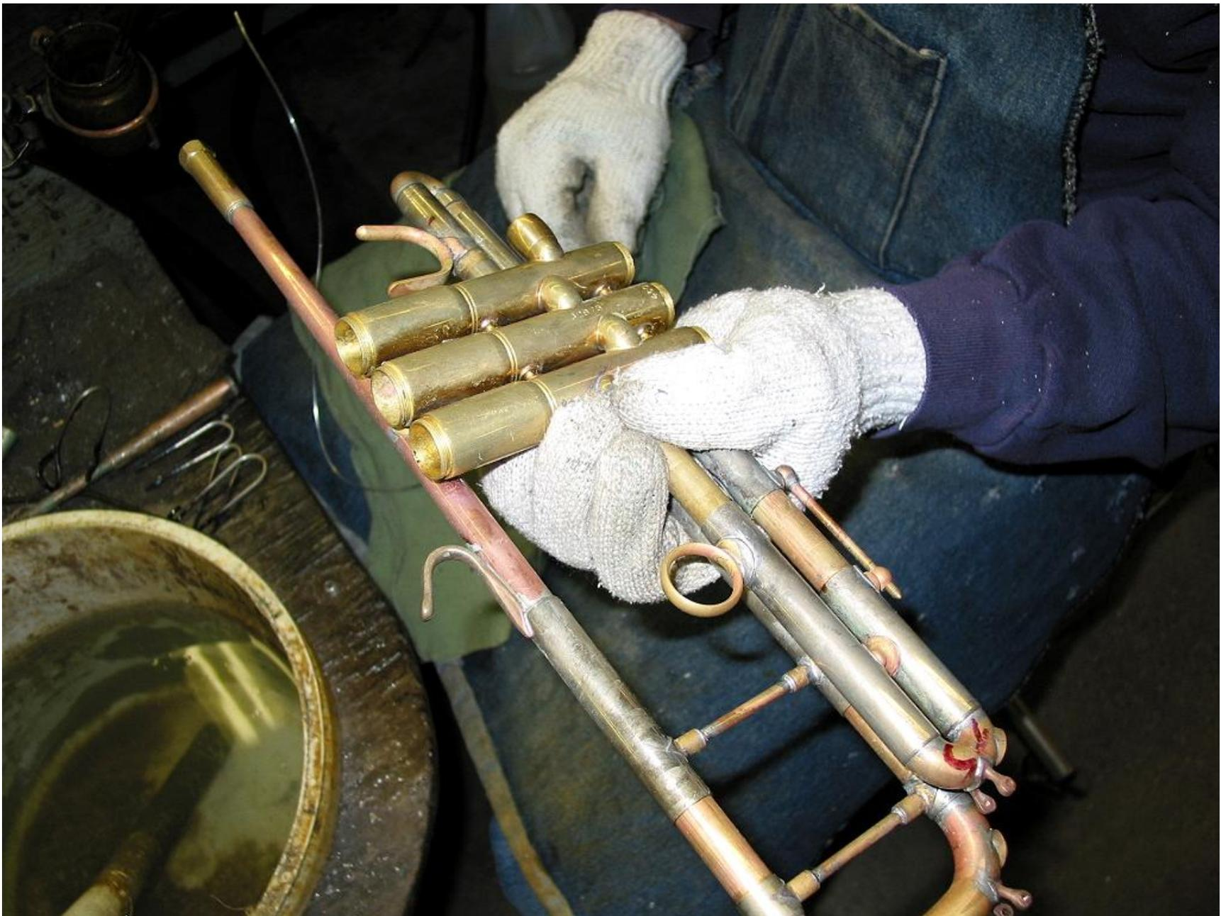
Some more assembly. Notice the lead solder wire? That is what holds a trumpet together as its melted and flows into all the joints and under braces. The copper leadpipe is a giveaway. Its a Guarnerius. This could be your very own Zeus Guarnerius being created.
