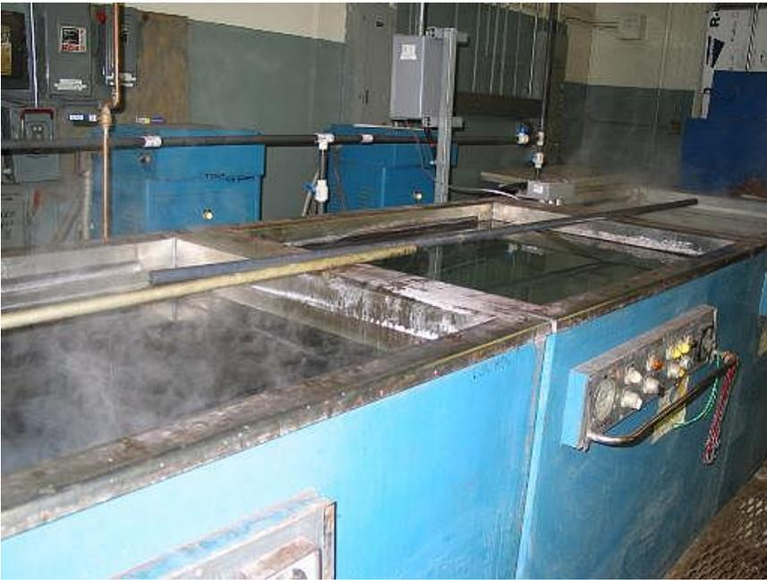
These are special ultrasonic cleaning tanks to completely degrease all parts. All traces of that greasy buffing compound must be removed in order for the lacquer or silver plating to stick to the instruments. This is a very important step. If an instrument is not thoroughly cleaned the finish will be shoddy.
