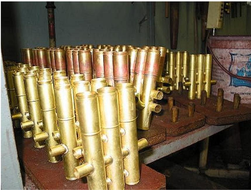
Valve sections after they have been soldered together.
