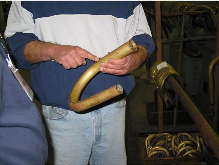
Explaining how a tar-like material has to be pored inside a tube before bending it so that the tube does not collapse in the process. Even though brass is a soft metal, a lot of pressure must be used to bend the tubes. Wrinkles or creases can not be allowed or you will complain as a customer. This is why the inside of the tubes must be filled with a rigid tar, which is melted and removed after the bending is finished.
