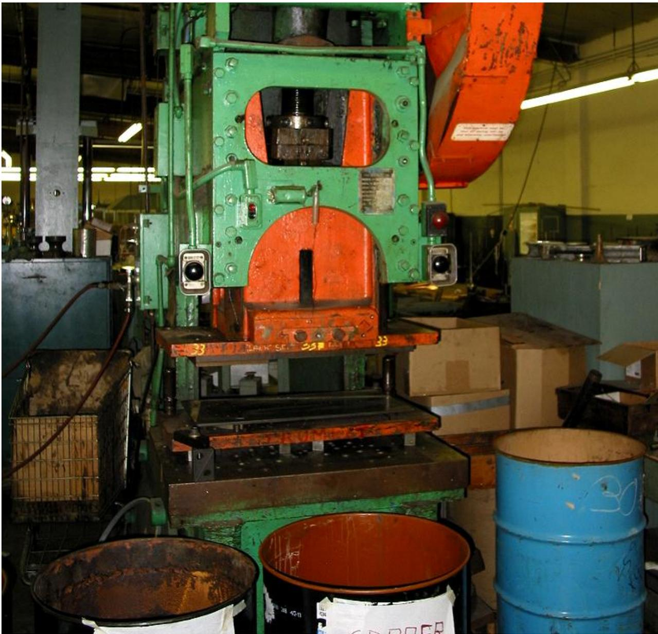
This punch press can either crush or cut. In this case it will cut out the exact size and shape of the sheet metal needed to make any bell. All in one motion. This step was done by hand with scissors in the past. The barrels in front is where they through the scrap brass or copper, after which it is sold to the scrap yard.
