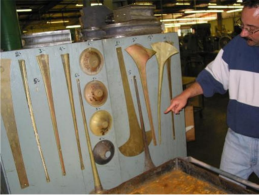
Showing the various stages of bell making. Two piece bells are on the left and single piece bells are on the right.
