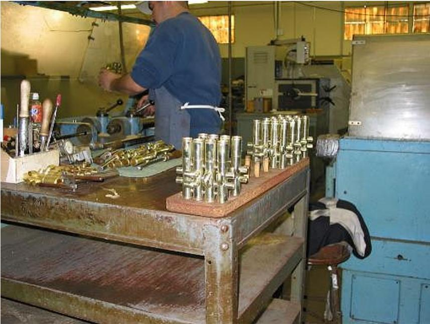
Here you see the valve sections after they have been soldered together with the slide tubes (knuckles) attached. The person in the background is performing a very interesting operation by which he draws steel balls through the casing knuckles and the piston valve ports in order to round out the channels in each valve.
