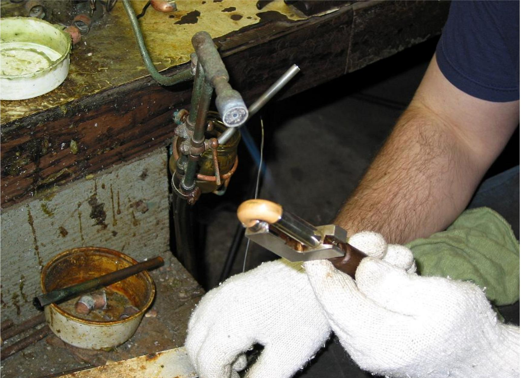
Various jigs are used to make the slides. They must be perfectly parallel to work smoothly. No crooked work here.
