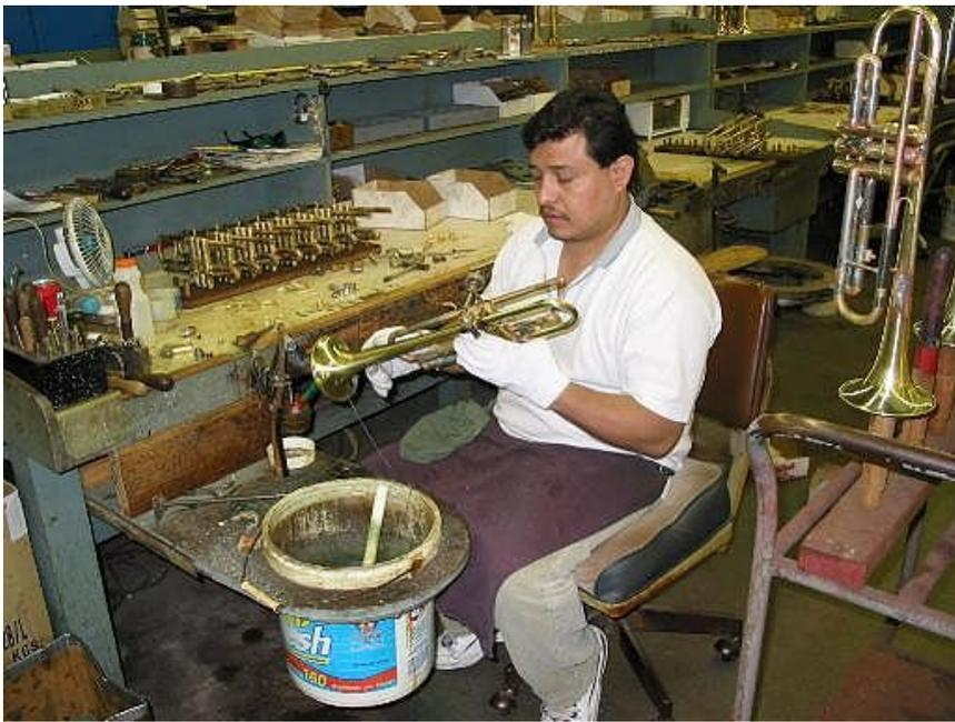
Soldering the bell to the valve section.
