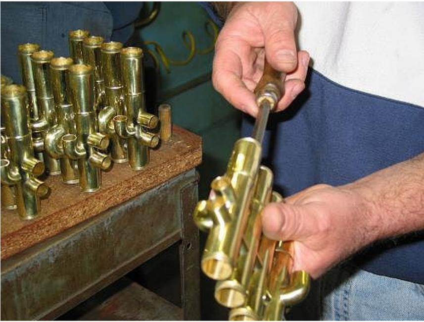
After the valve casings are soldered together they must be de-burred so that the insides of the casings are perfectly smooth with no protruding pieces of metal.
