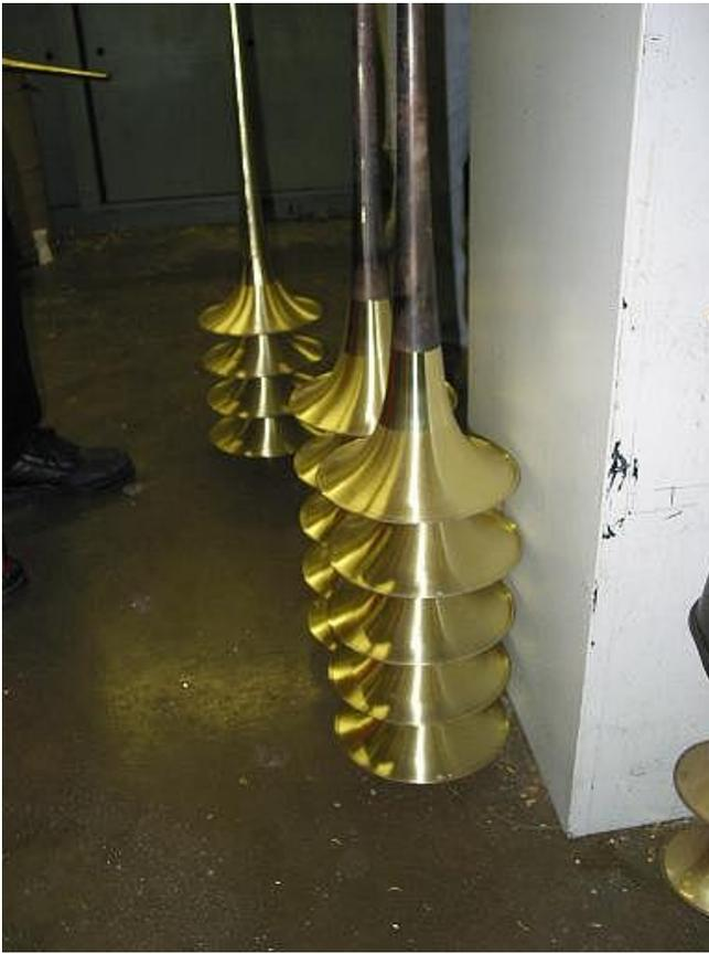
Finished two piece bells. You can see the color variation between the two pieces, the flare and the stem.
