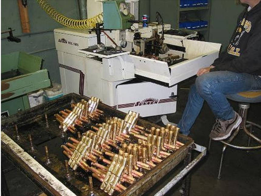
Initially, the valve casings are reamed to size by that white boring machine in the background. Later after the instrument is assembled and is ready to be fitted with valves, each piston is hand lapped in its own casing for that perfectly tight fit with very close tolerances. Each valve must be lapped to conform to its own valve casing.
