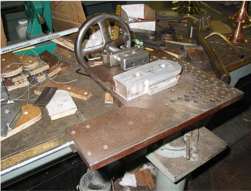
This is the manual bending jig used make the curve in the end of trumpet bells.
