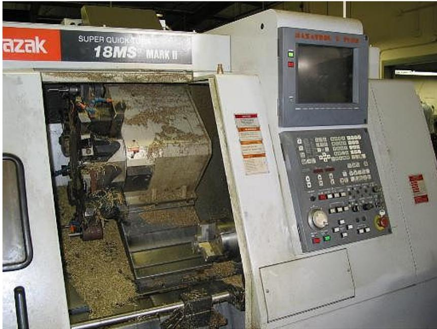
One place where computer precision does come in handy is when making mouthpieces. Mouthpieces are made on this computer controlled machine that is extremely accurate and cuts the same shape consistently every time
