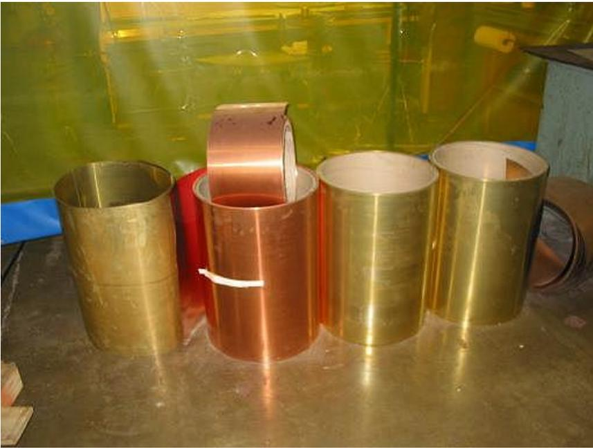
The various sheet metal used for bells. Initial bell shapes will be cut from this sheet metal just like in the garment industry.
