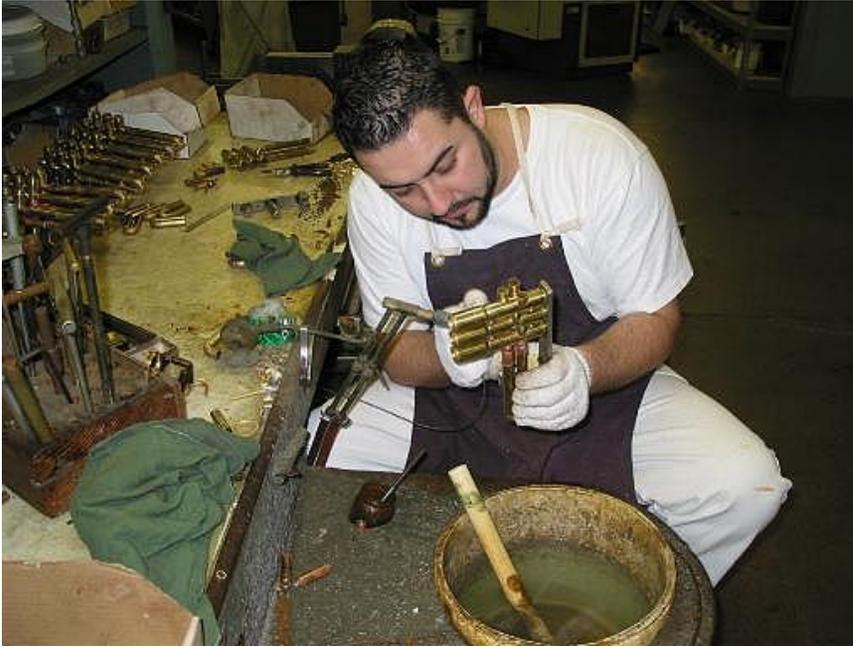
Soldering the initial slide tubes to the valve casings.
