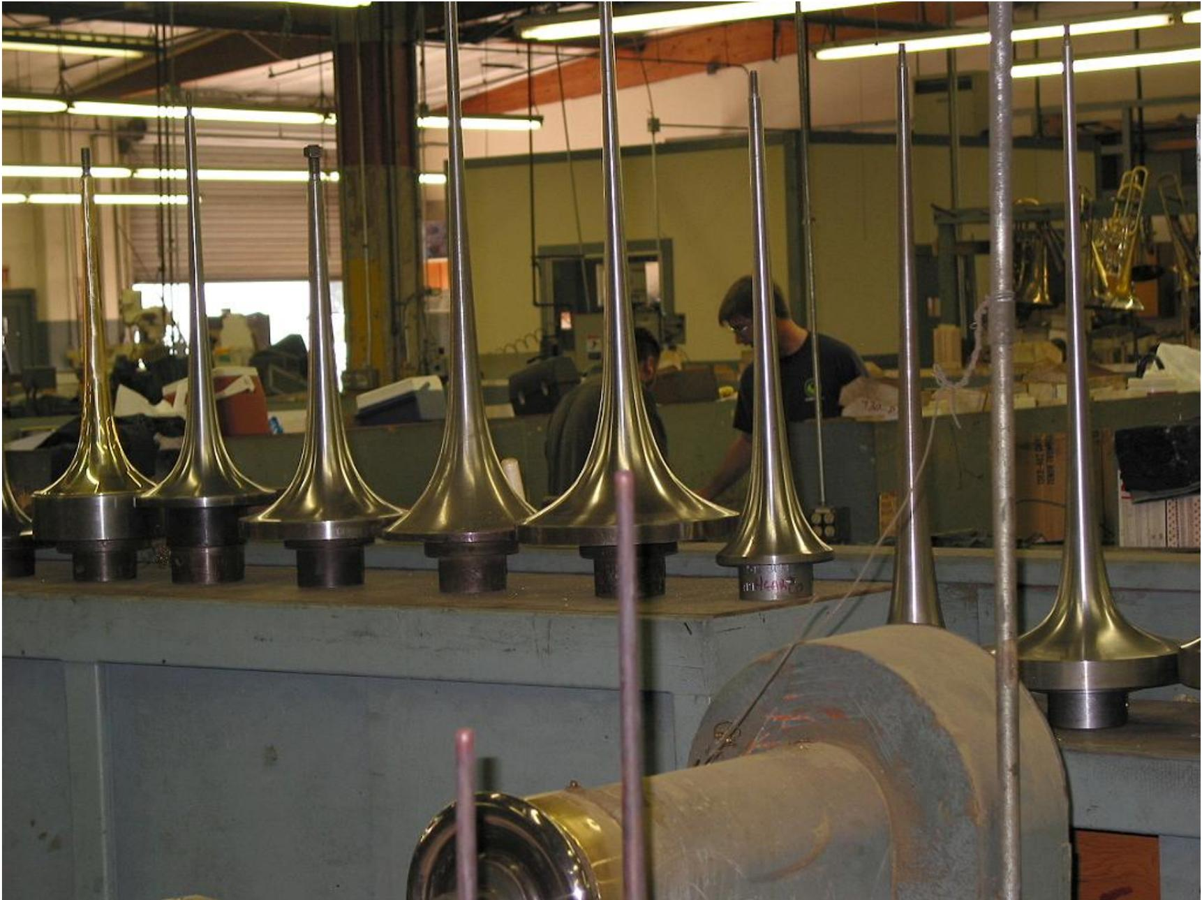
These are the various steel mandrels use to spin bells by hand on a lathe. Each model instruments needs
