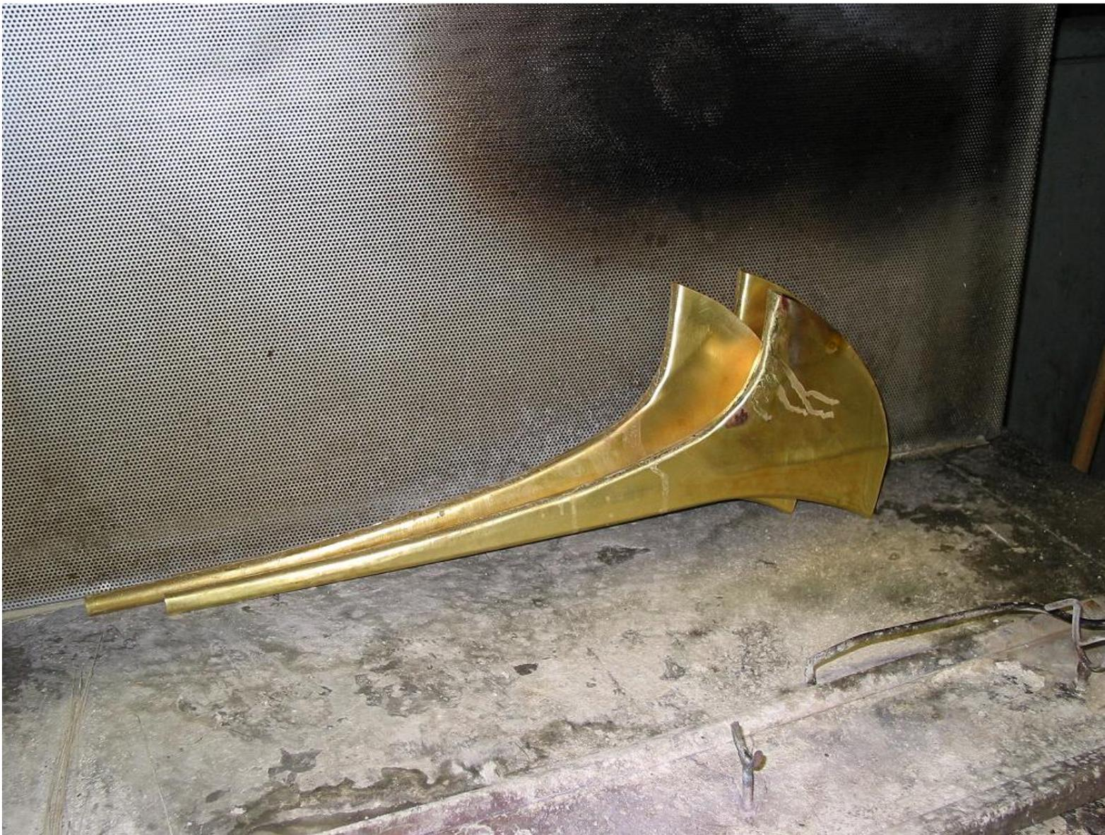
This is a chamber in which they use a torch to make the bells red hot again to "anneal" them. High heat softens brass so that it can be worked easier. Hammering or burnishing hardens brass once again. This is called work hardening. For this reason the bells need to be heated up to certain temperature to be "annealed" many times during the course of their construction and forming.
