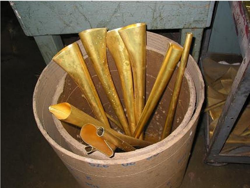
The bell stems of two piece bells waiting to be soldered to the flare part. Two piece bells are made of two parts, the bell flare and the bell stem. These are the stems.
