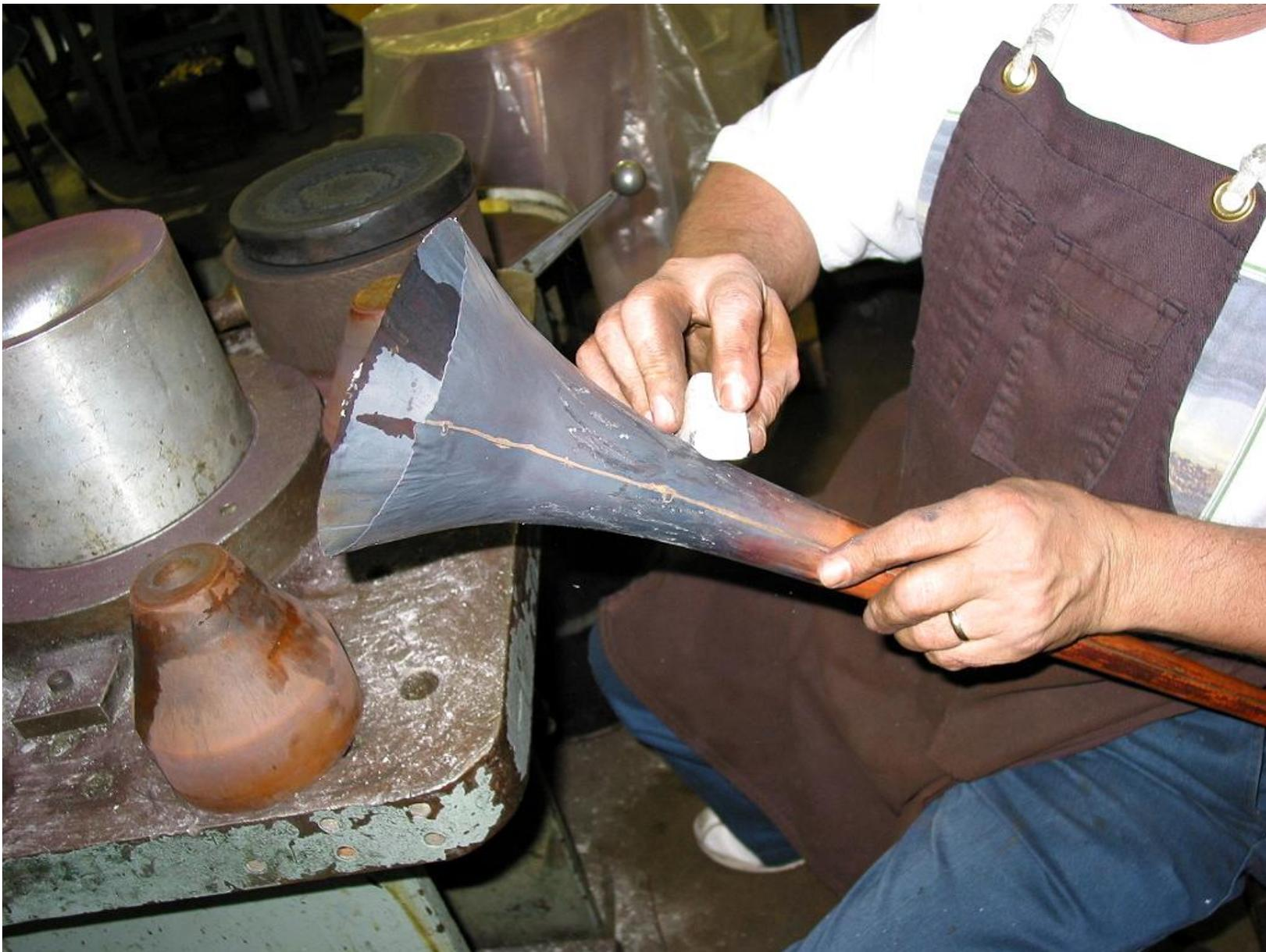
Getting the bell material lubricated before its put into the brass for forming.
