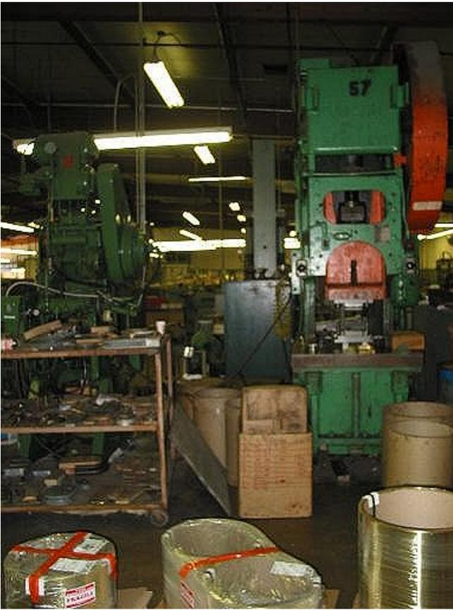
Notice those big green monsters in the back? They are punch presses which come down with several tons of pressure on pieces of brass and form them into parts such as braces that hold the instruments together.
