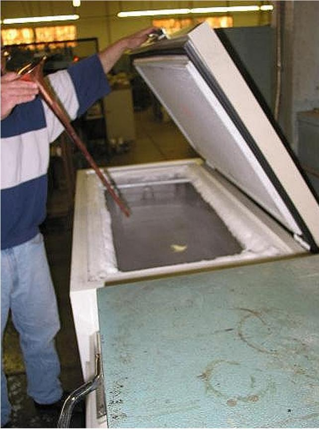
Its cold in there. This is where the bells are placed in order to freeze the soap and water mixture inside the bell. The mixture freezes but as much a pure water would. This way it does not crack the thin wall of the bell. The soap and water mixture freezes just enough to stop the tube from collapsing when placed into the bending jig shown below.
