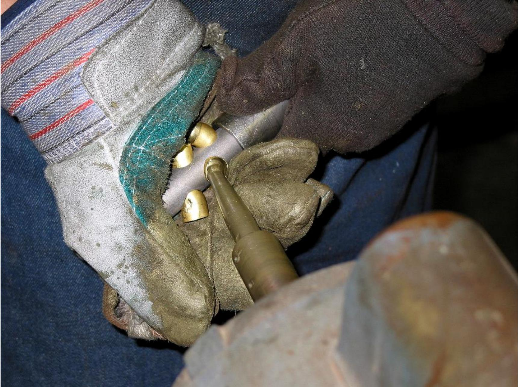
Ever wonder how they make the valve section the proper bore size? The "ball" it out with the proper size ball. The little connector tubes coming out of each valve casing are called knuckles and this is how
