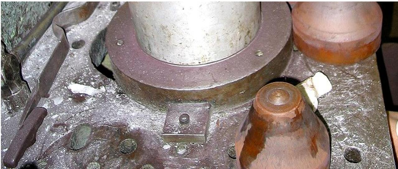
Notice the cone shaped objects on the right side of the table. These are inserted in the press above, which comes down with force and forms the bell flare to the shape of the bottom piece. This is still part of the initial forming process.
