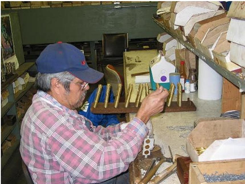
Placing the individual valve casings in a soldering jig to be soldered. You can imagine that everything must be perfectly aligned before it is soldered. The jig helps with this alignment.
