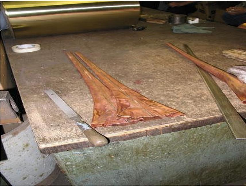
Sheet copper has been cut to shape and then soldered together down the middle. You can see the seam going down the length of the bell. This process is very much like making clothes. They use a pattern to cut the sheet metal to the proper shape. Its hard to believe that these will be beautiful copper trumpet bells. These will be one piece bells as opposed to the two piece bells pictured below.
