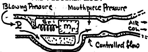
Controlled our flow enters our colum thru the reed aperture. FLOW = A. (1-P)
