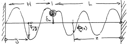
Here, the left and right strings have their displacements  $\psi$  and  $\phi$  defined in terms of the (known)k and a sine function measured in from the "request") end via the coordinates y and z. The displacement of the hammer mass M is denoted by  $\delta_{\rm L}$ . That is
