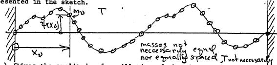
Here  $\psi(x_0)$  gives the amplitude of oscillation of the element of mass m whose "address" along the chain is x. The sequence of x can be discrete or continuous. In the latter case  $m_{\mu} = \mu(x_{\mu}) dx$ , the mass of a short piece of chain having length dx and local linear mass density  $\mu(x_{\mu})$ .
