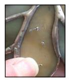
You may find small pieces of solder stuck to the glass. You can easily remove these using your fingernail, or 000 steel wool. Be careful not to scratch the glass.
