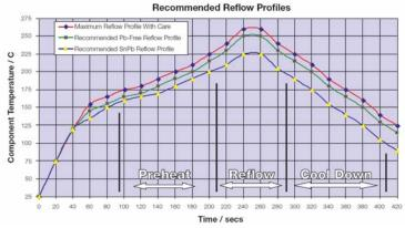
Figure 30: Typical Oven Program for Ceramic Capacitors
