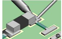
Figure 34: Fixing the Second Side of a Component
