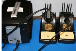
Figure 1: OKI Soldering/Desoldering Station
