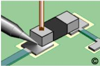
Figure 33: Fixing One Side of a Component
