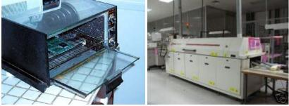
Figure 29: Soldering Ovens
