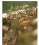
Figure 35: Cracked and Cold Solder Joint
