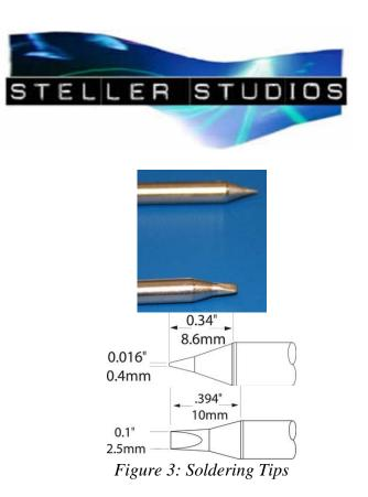
Each tip can be used for a variety of tasks. The smaller tip is best used on smaller components where less heat and more precise heating is required. Example of areas to use the conical tip are SMT parts, Dual in Line Packaged (DIP) integrated circuits (IC's), and small leaded (<0.05" diameter) components.
