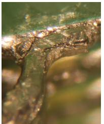
Figure 22: Cracked and Cold Solder Joint
