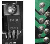
Figure 5: Example of TO220 and Larger Connector Solder Pads
