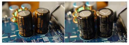
CAPACITORS ON FAILED MIDPLANE CAPACITORS ON NEW MIDPLANE Figure 21: Over Heated Capacitors
