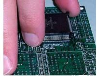
Figure 28: Position the Component
