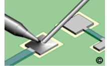
Figure 32: Adding Solder to One SMT Pad
