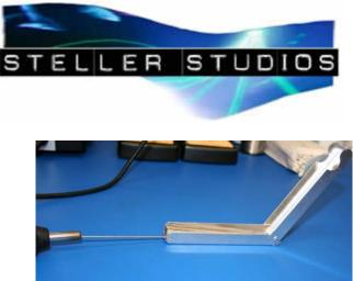
Figure 8: Using the Desoldering Iron Cleaning Tool
