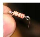
Figure 17: Coiled Resistor Leads to Reduce Vibration Shearing
