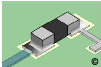
Figure 35: The Soldered SMT Component
