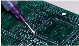
Figure 27: Appling Solder Paste By Syringe
