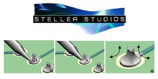
Figure 41: Proper Soldering Technique.
