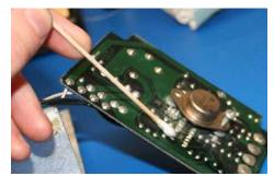
Figure 23: Re-Clean the Desoldering Area
