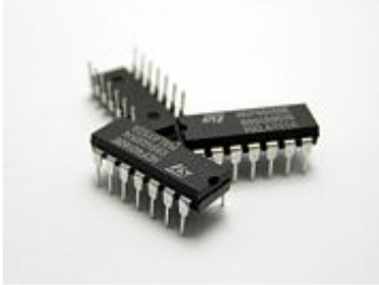
Figure 3 DIP (dual in-line package)
