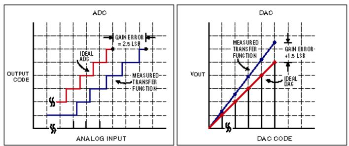
Gain error for an ADC and a DAC.
