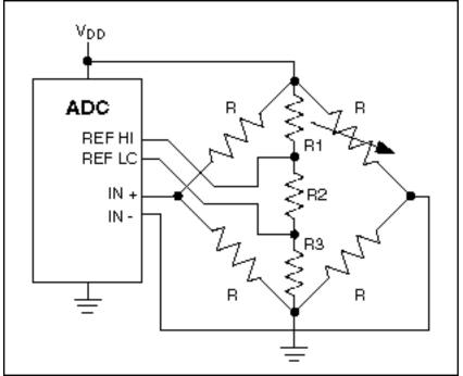
Ratiometric measurement using resistive bridge network.
