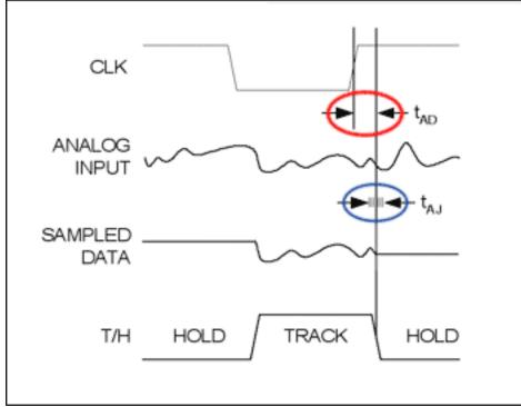
Aperture delay (red) and jitter (blue).
