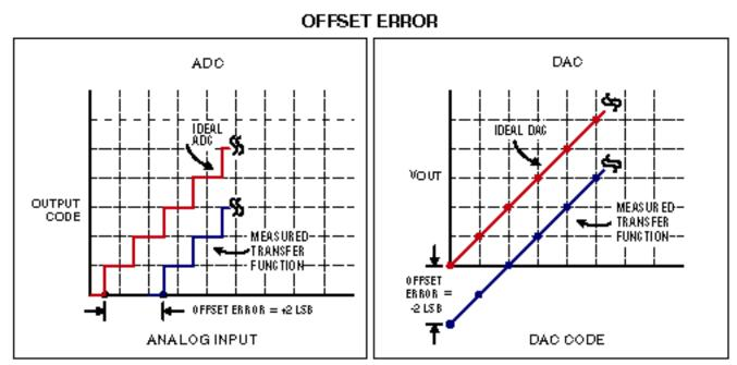
Offset error for an ADC and a DAC.
